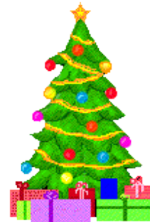
Fig. 1. General structure of tree-formed SML and according verification data. The star represents the root of the tree stored in a verification data register. Components (code and/or data) are indicated by packets at the leaves. Measurements hashes of the components are indicated by slip knots. Inner nodes (coloured balls) transport verification information upstream to the root. The golden lines hint at the traversal of the tree for validation, explained in more detail in Section IV.
